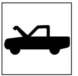
1. Pull the handle with this symbol on it. It is located inside the vehicle to the lower left of the steering wheel.
